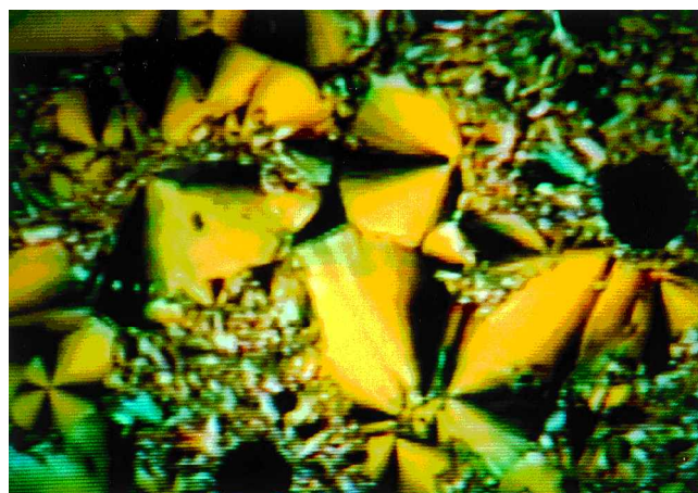
Figure 3. Microscopic texture observed for the M phase of the dodecyl member ( n=12 ) of series V at 94^\circ\text{C} .
